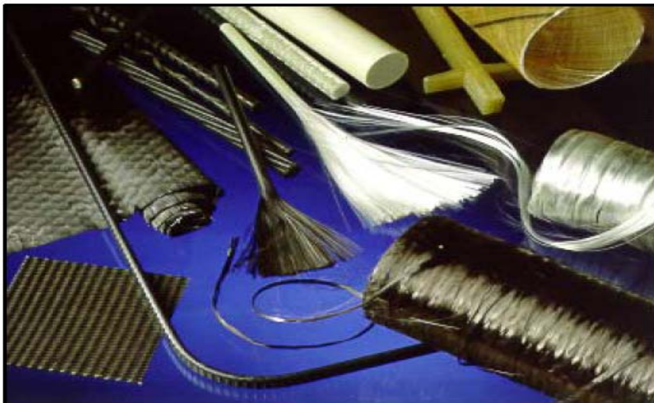
Fig. (2-2): FRP Products Currently Used for Reinforcement or Rehabilitation of Concrete Structures, [ISIS-EC-2, 2006].
